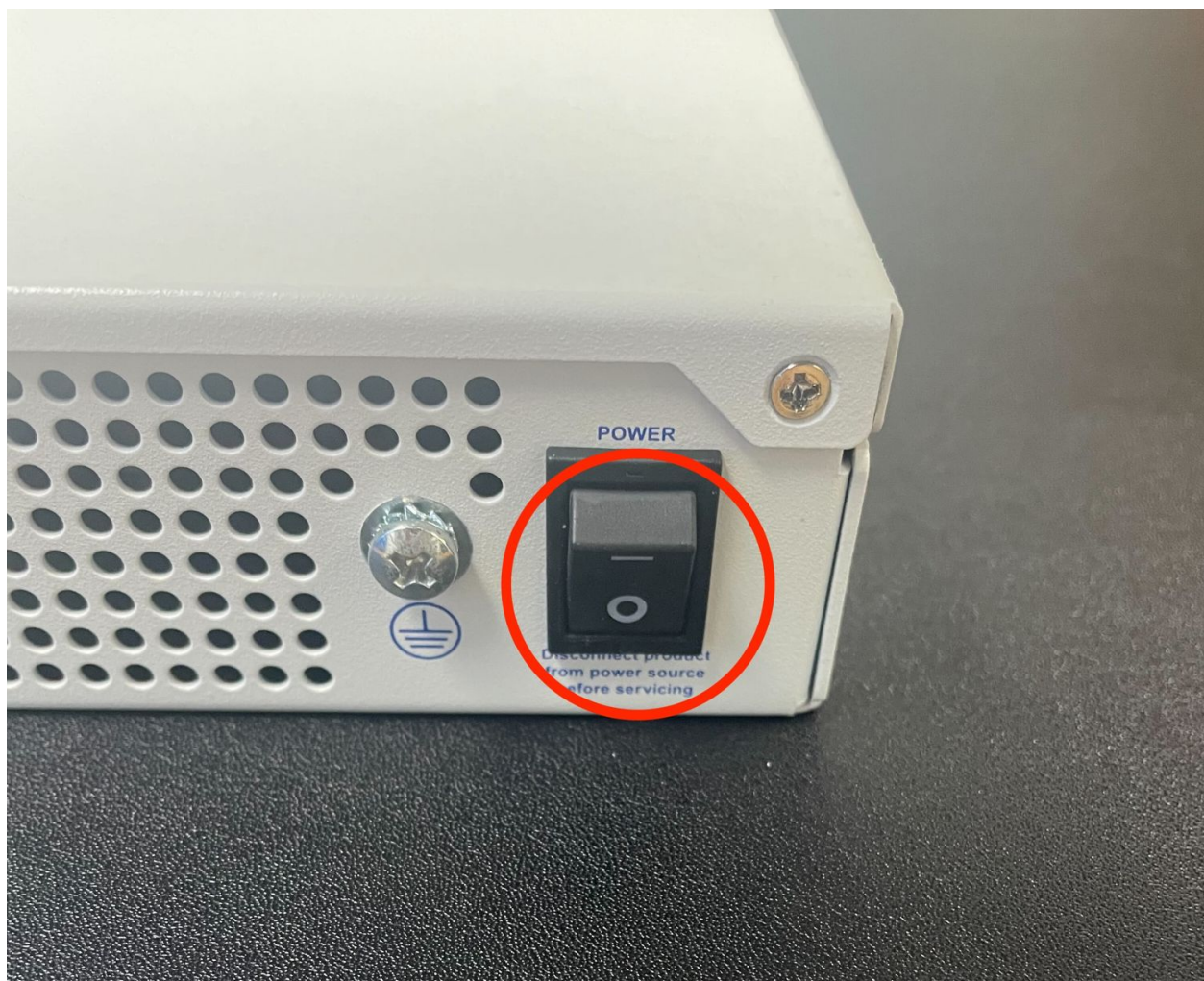
Fig. 21: Power switch (circled) in the off position
