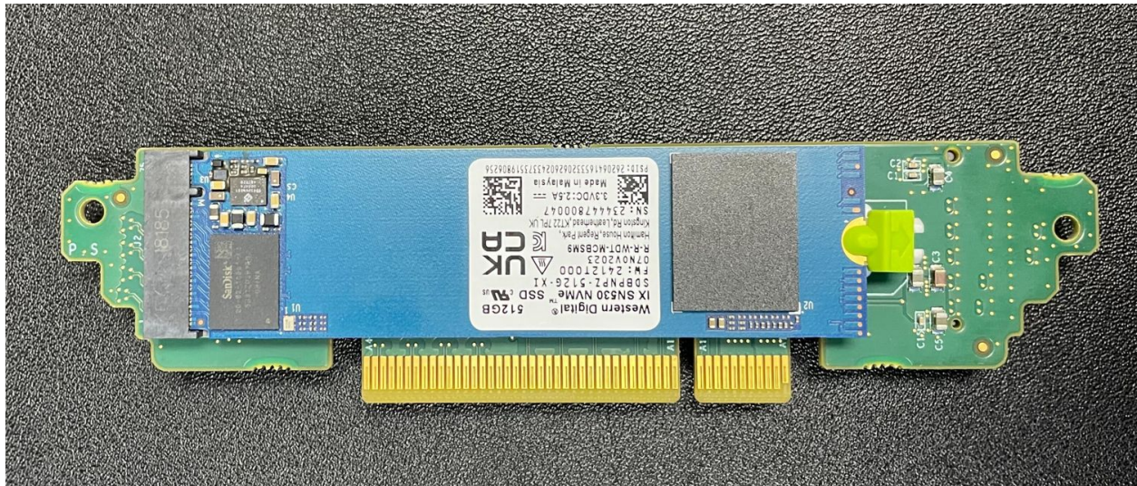
Fig. 45: M.2 NVMe riser card slot 1 with the stock SSD installed
