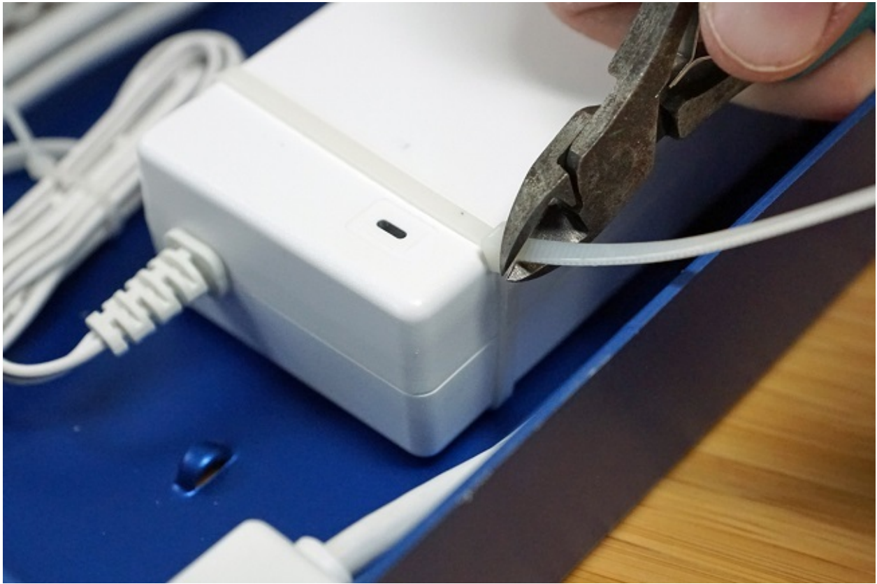
Fig. 14: Cut the Excess Cable Ties
