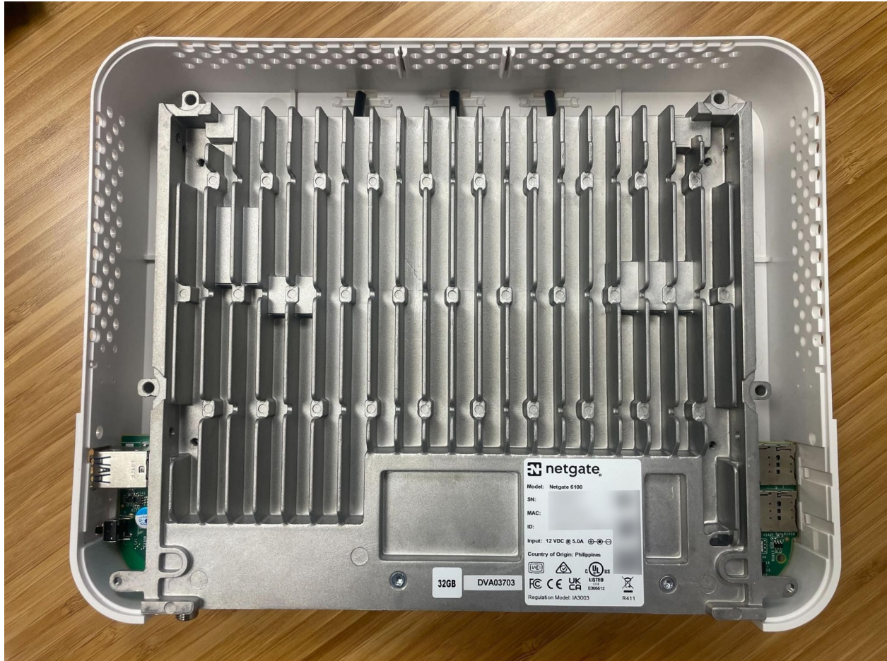
Fig. 27: Netgate 6100 with bottom panel removed
