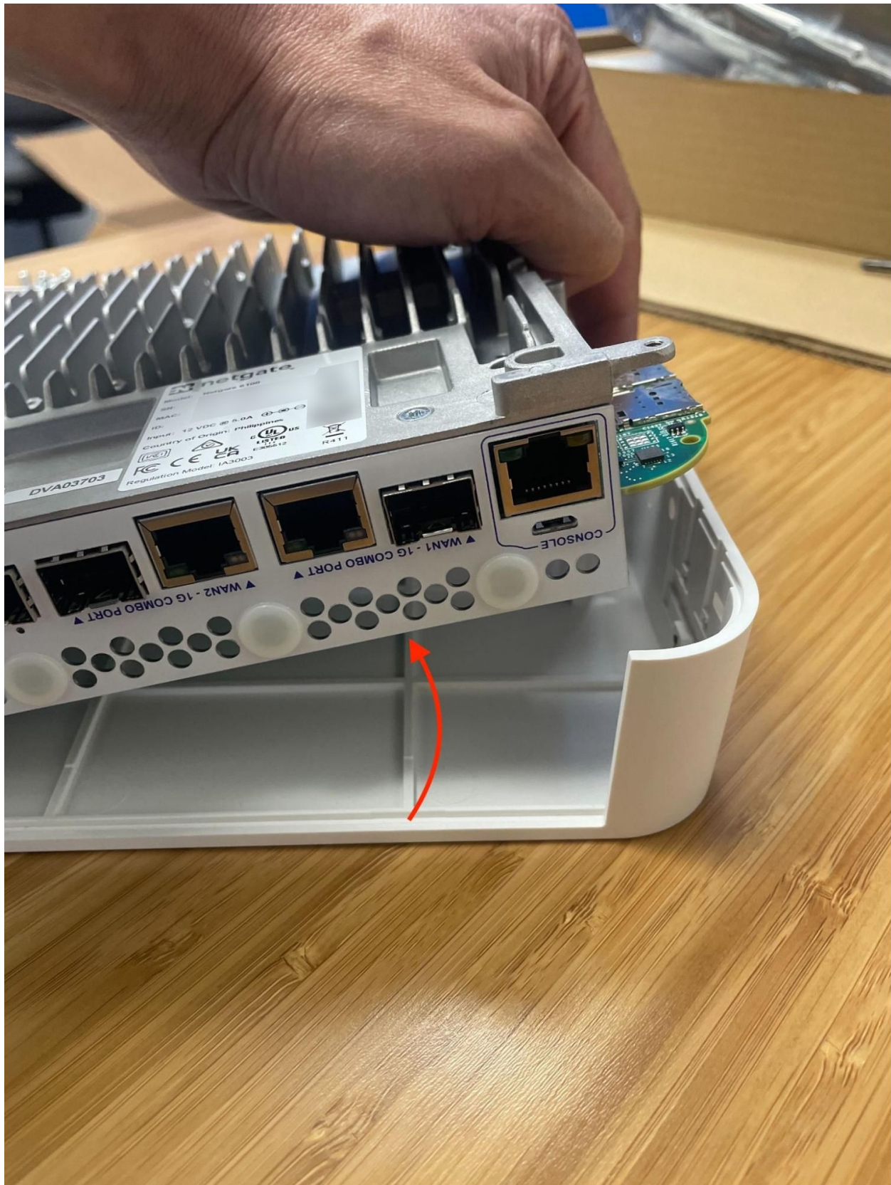
Fig. 29: Removing the Netgate 6100 chassis from the lid
