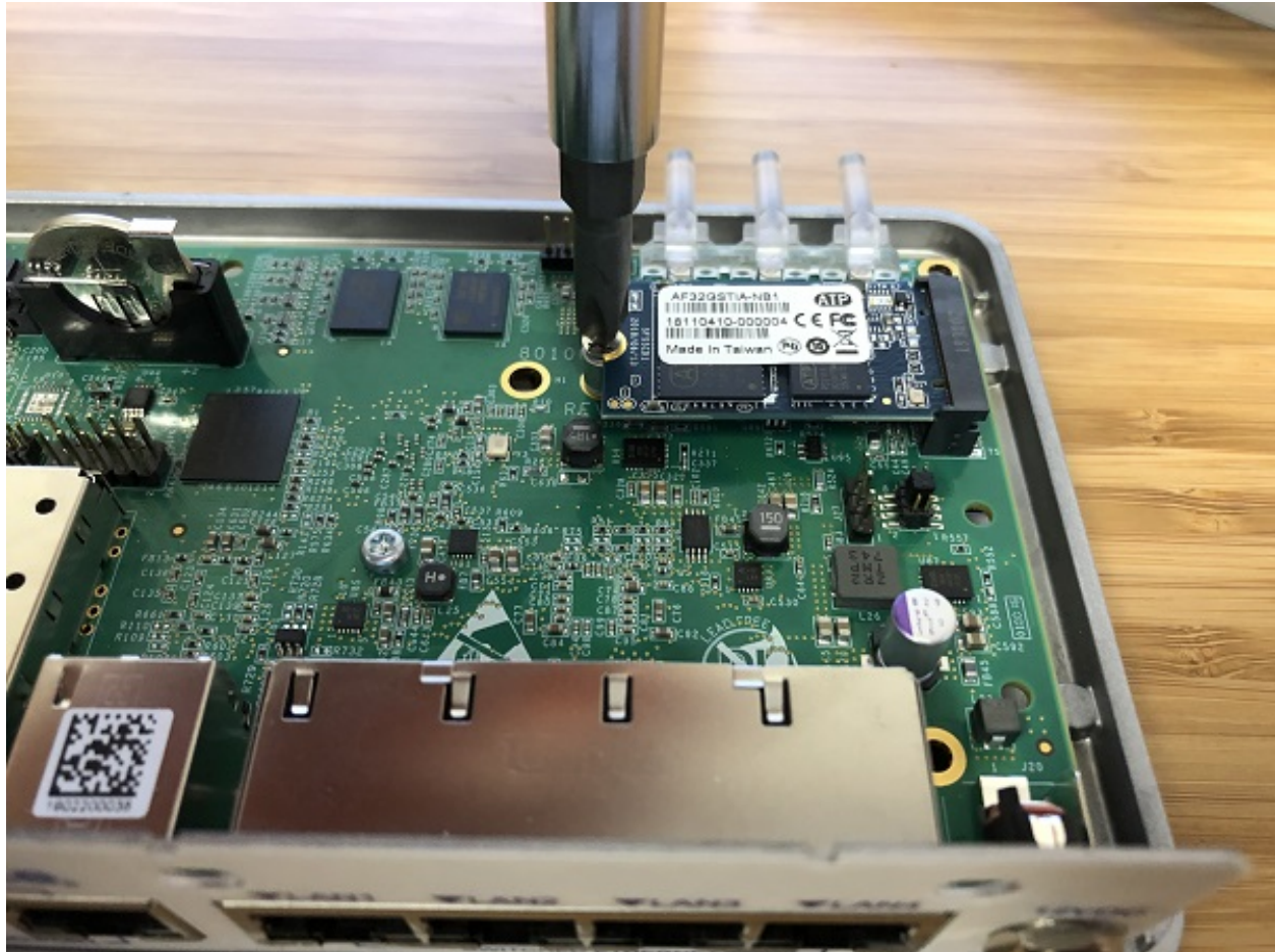
Fig. 4: The M.2 SATA Drive Installed
