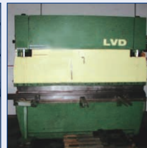
Kantbank/Hydr. Pressbrake LVD, type PP80/25, 80 ton x 2.500 mm.
