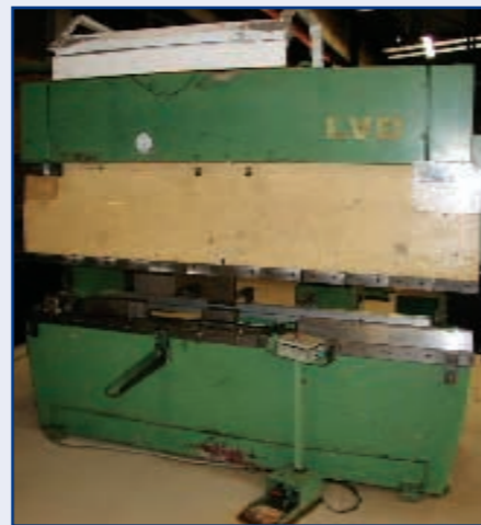
Kantbank/Hydr. Pressbrake LVD, type PPNMZ80/30 NC, cap. 80 ton x 3.000 mm, besturing Cybelec.
