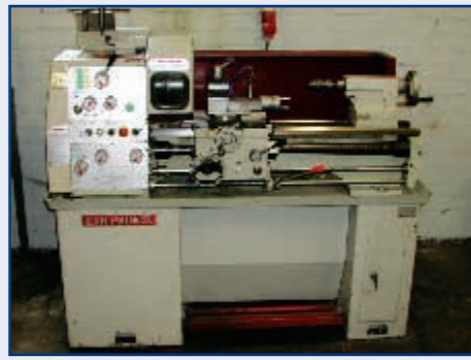
Draaibank/Lathe ENR PRINCE, cap. 600 mm t.d.c. x 100 mm c.h.
