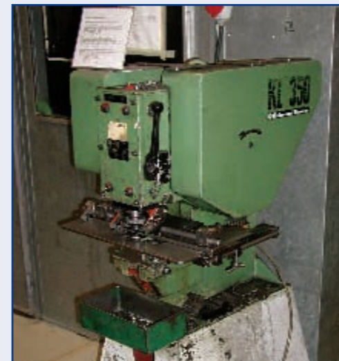
Gecombineerde ponsknipmachine/ironworker MUHR UND BENDER, type KL 350, pons ø 28 in 10 mm, ø 23 in 12 mm.
