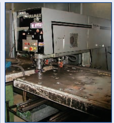
Ponsmachine/Punch PULLMAX, type 210 DMC, stempel diam. 210 mm, besturing Facit N 1060 + kogeltafel.
