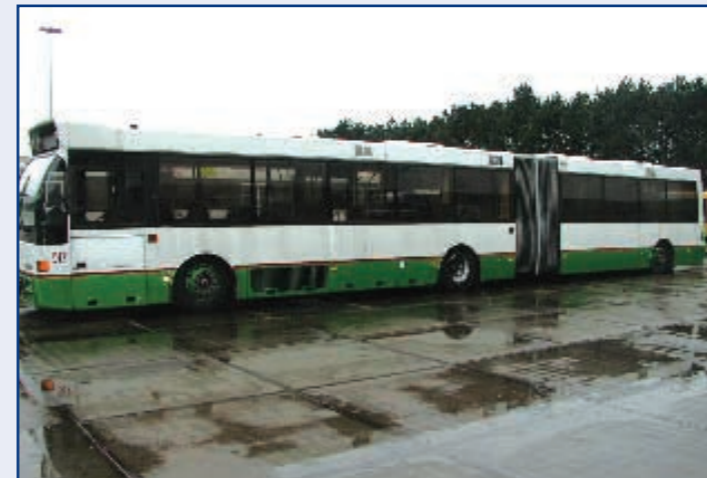
Gelede bus/Articulated Bus BERKHOF, type B10 M-A Articulated, v.v. VOLVO motor.
