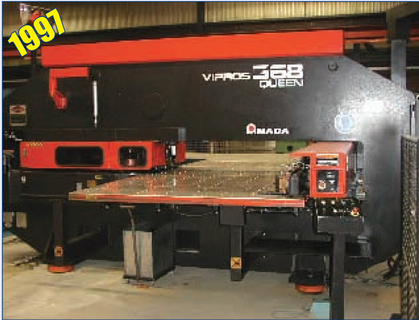
CNC Revolverponsmachine/CNC Turret Punch AMADA, type VIPROS 368 QUEEN (1997), CNC gestuurd, stanskracht 294 KN, 45 revolverposities, X-as = 2.000 mm, Y-as = 1.525 mm.
