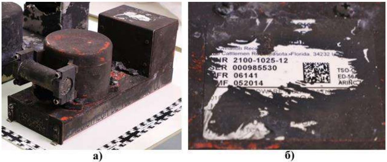
Fig. 31. The L3 FA2100 CVR: a) the general view; b) the unit data plate
