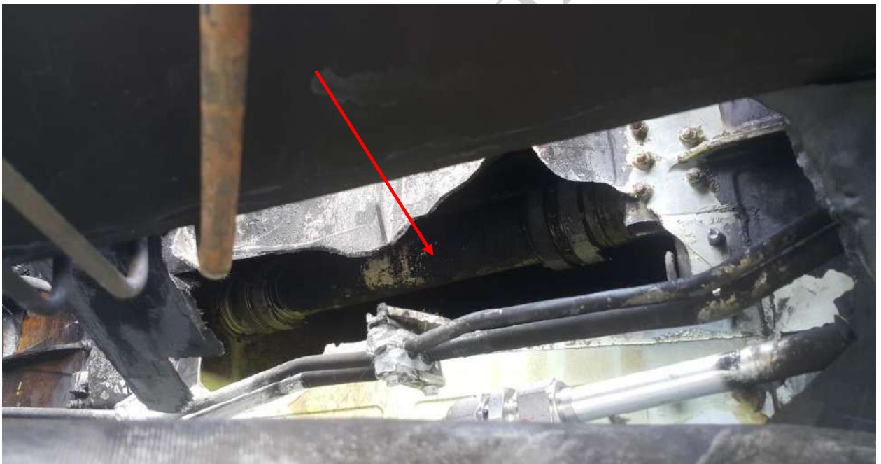
Fig. 8. The hole in the right wing spar web at the cylinder mounting location (pointed with arrow)
