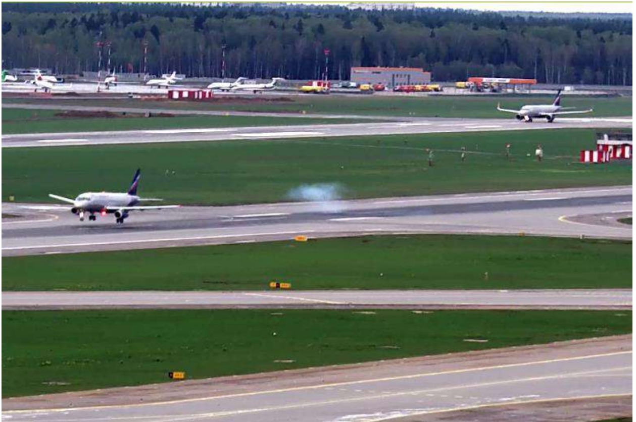
Fig. 34. The aircraft separation (the bounce) off the RWY
