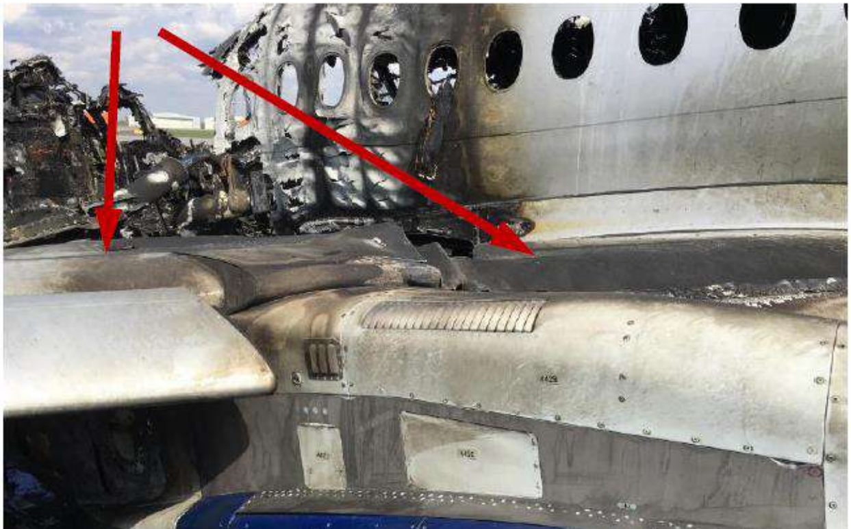
Fig. 9. The destruction of the right wing adjacent to ribs 3-4 in between the fuselage and engine pylon
