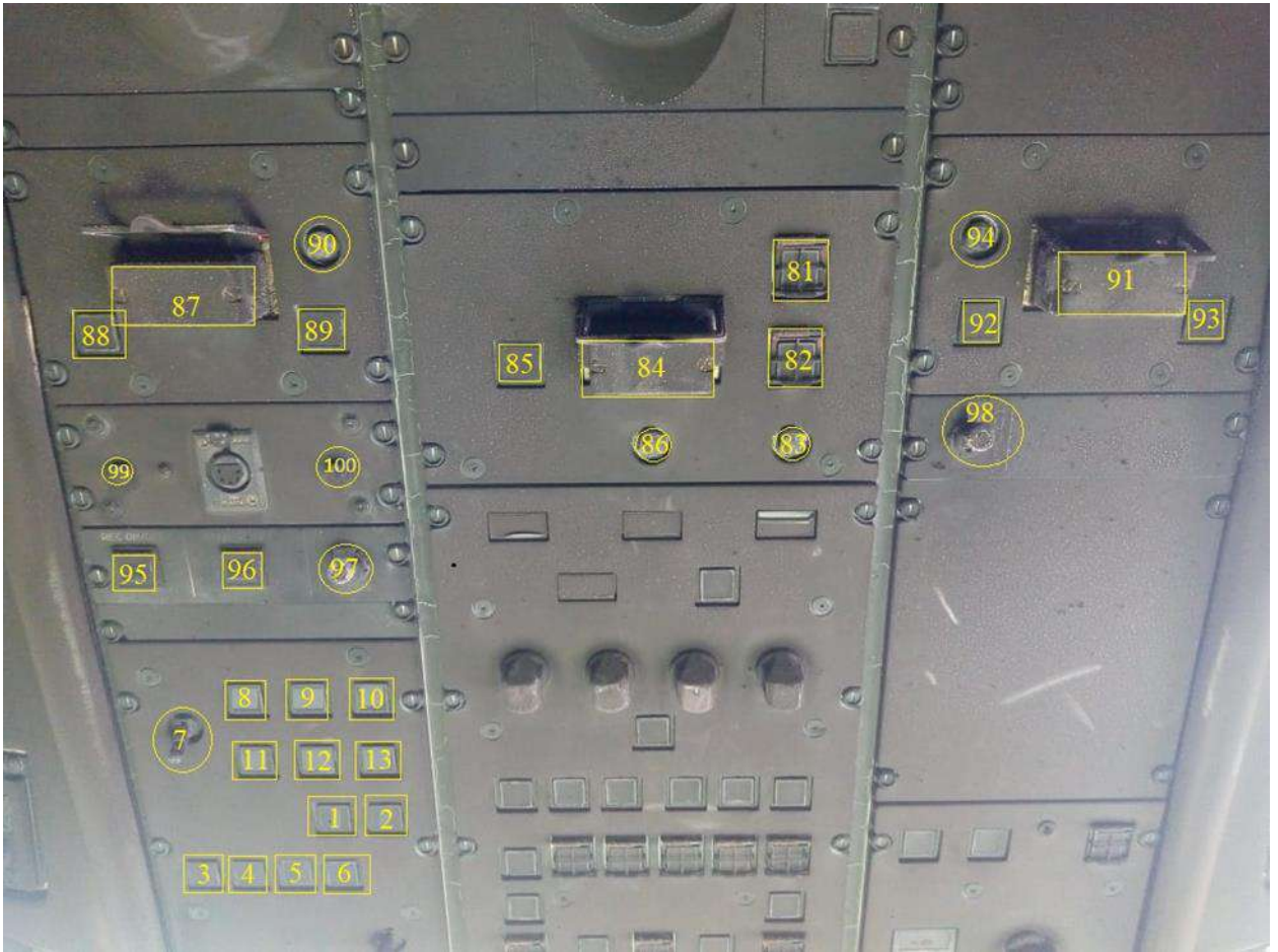
Fig. 21. The post-accident position of the ENG FIRE and APU FIRE switchlights
