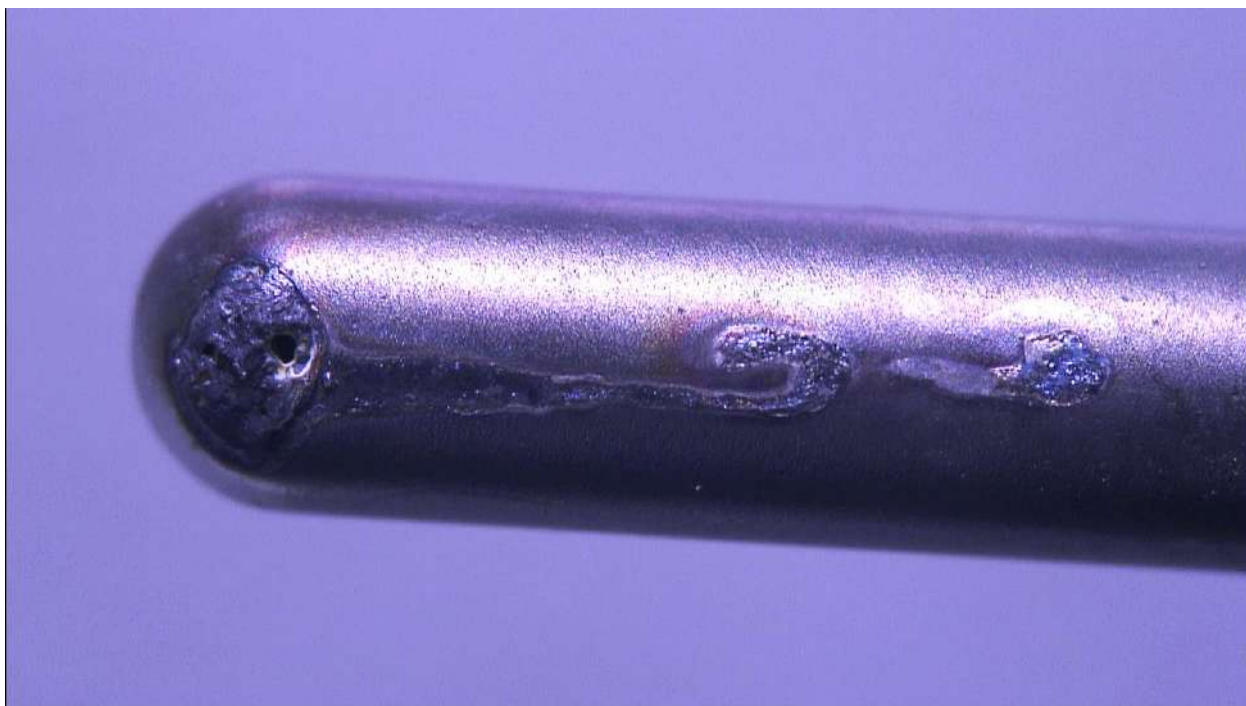
Fig. 25. The lightning exposure traces on the right ice detector
