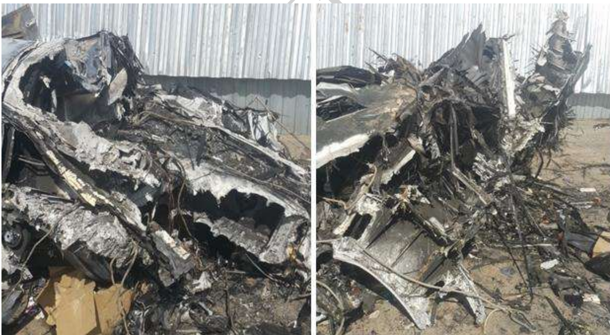
Fig. 6. The post-accident exterior of the vertical and horizontal parts of the empennage (the picture was taken at the storage site)
