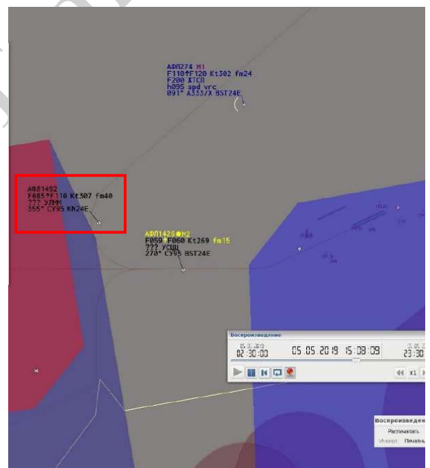
Fig. 161. The AFL1492 flight (highlighted with red color), the point of the atmospheric electricity strike against the aircraft
