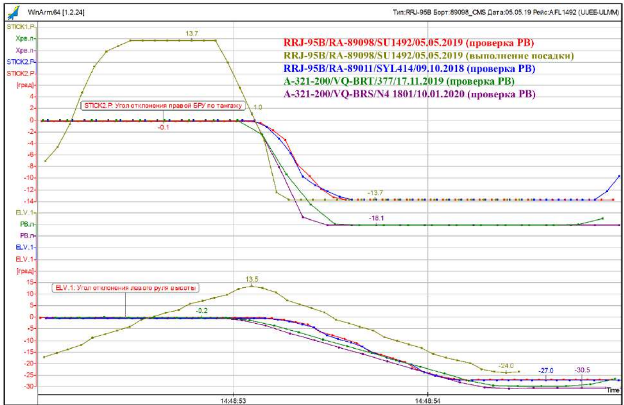
Fig. 171. The comparison of the elevator travel rates at the dynamic sidestick inputs (the time is relative on the Figure)
