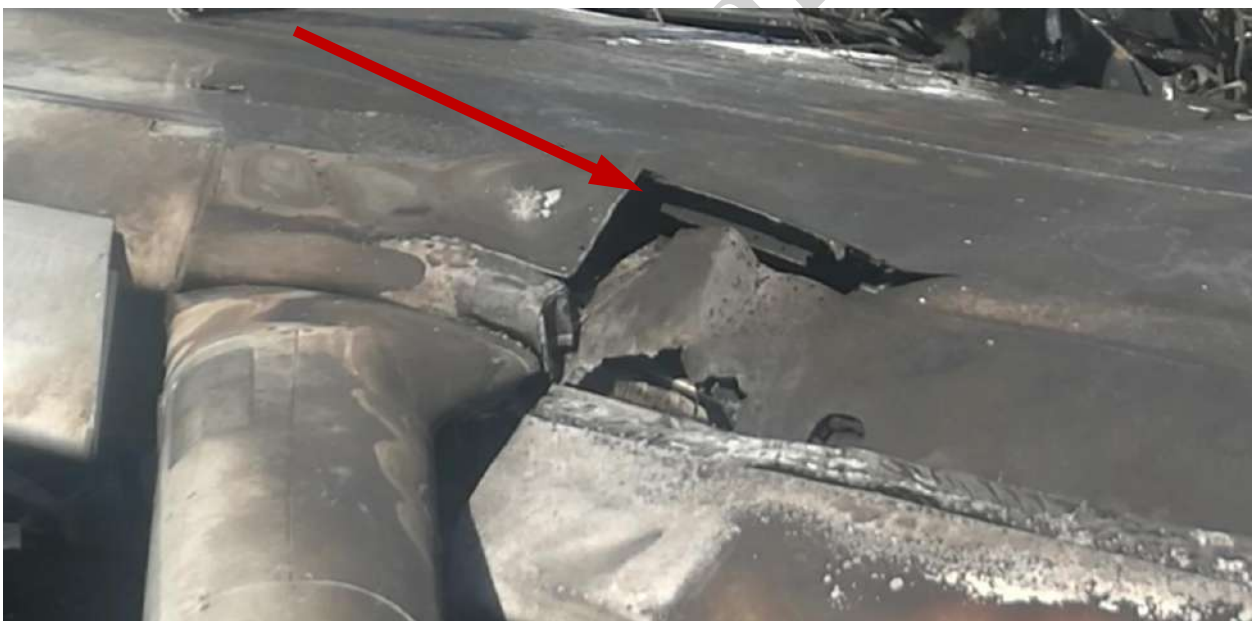
Fig. 10. The destruction of the upper panel and the fore spar of the right wing adjacent to ribs 3-4 in between the fuselage and engine pylon
