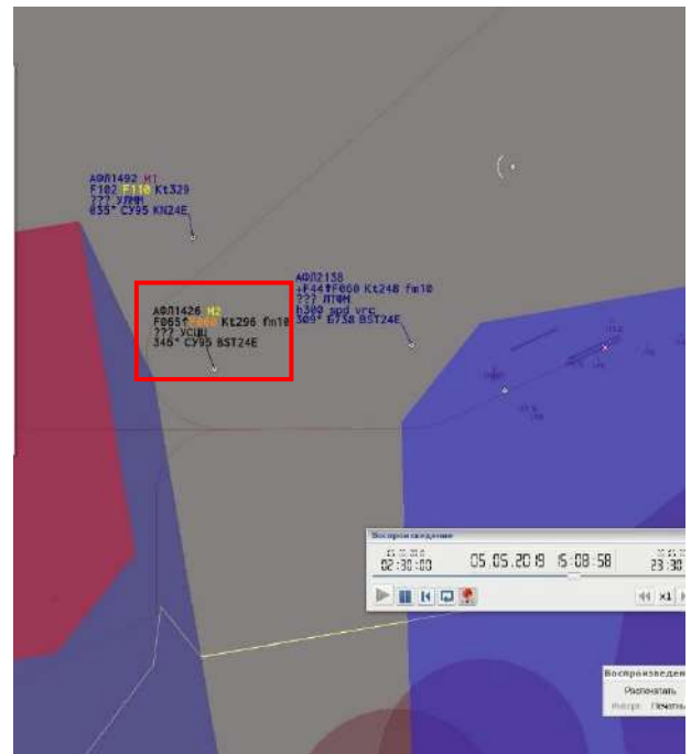
Fig. 163. The AFL1426 flight (highlighted with red color), the point of the closest aircraft approach to the thunderstorm front
