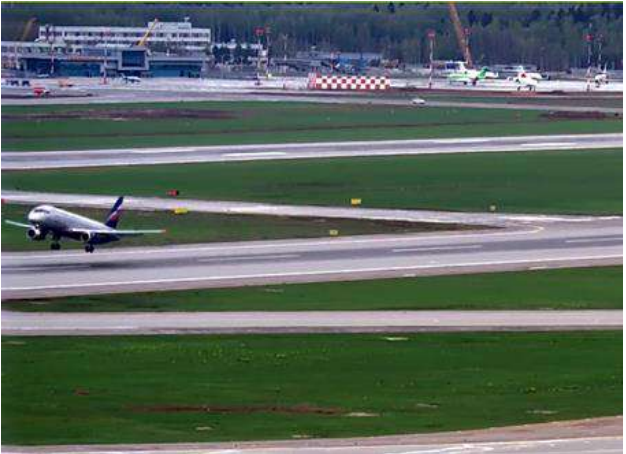
Fig. 36. The aircraft bouncing off the RWY after the second touchdown
