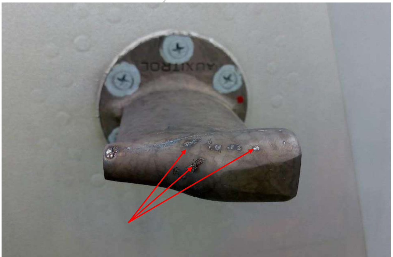
Fig. 24. The lightning exposure traces on the right temperature sensor
