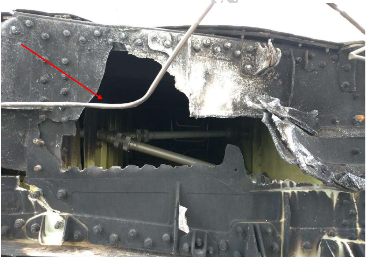
Fig. 12. The hole in the left wing spar web at the actuating cylinder mounting location (pointed with arrow)
