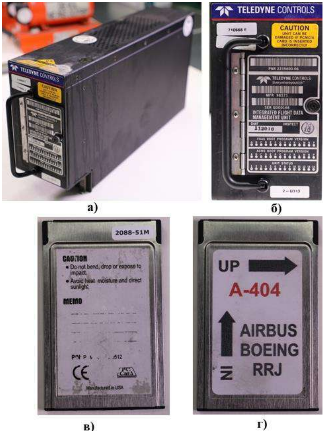
Fig. 32. The IFDMU operational data collecting device with the PCMCIA flash card (# 2088-51M): a) the general view of the unit; б) the unit data plate; б) and r) the PCMCIA flash card (# 2088-51M) on both sides
