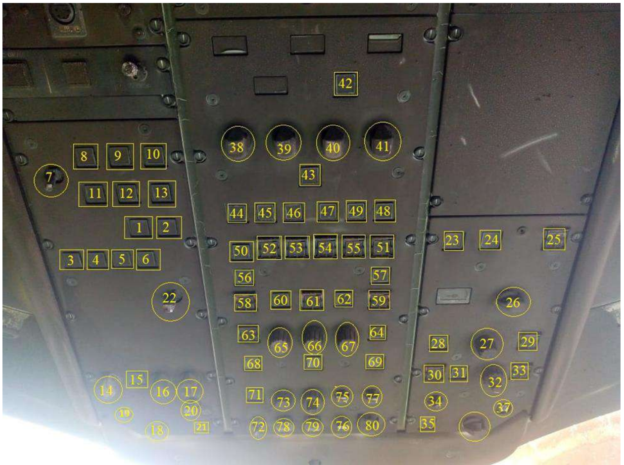
Fig. 22. The post-accident position of the batteries switches
