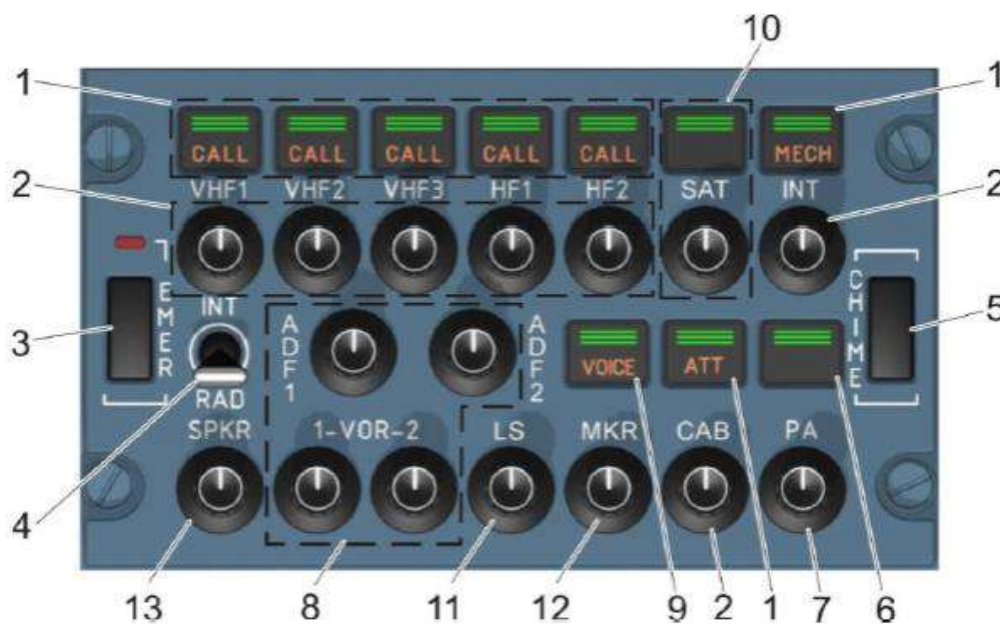
Fig. 134. The exterior of the ACP control panel
