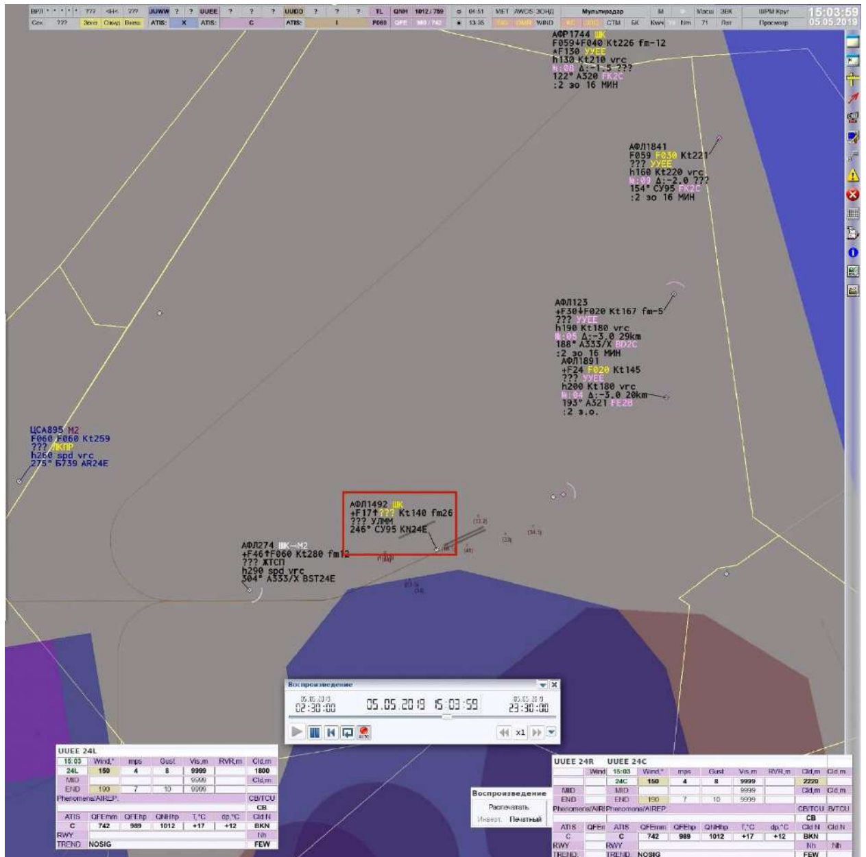
Fig. 178. The SYNTEZ-AR4 ATC automated complex indication at the Radar controller's duty station at 15:03:59 when receiving the AFL1492 flight for control (the aircraft data block is outlined with the red rectangle)
